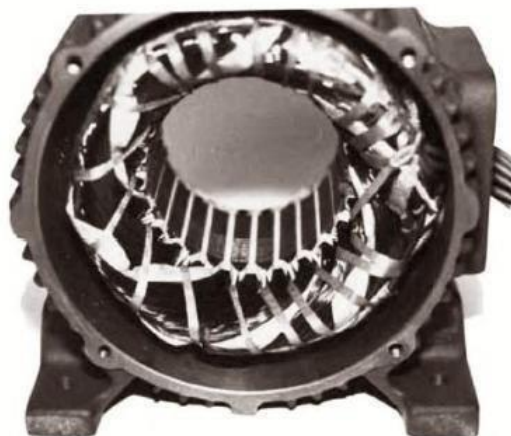
Fig: The stator of a typical induction motor showing the stator windings
