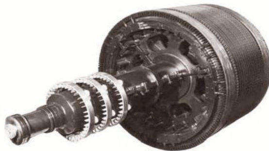
Fig: Typical wound rotors for induction motors. (Notice the slip rings and the bars connecting the rotor Windings to the slip rings)
