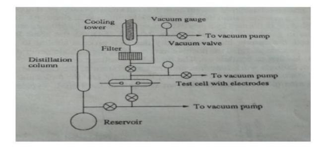
The general impurities in liquid dielectrics are dust particles which cane removed by the process of filtration, gas bubbles and moisture are other impurities which can be eliminated by distillation and degassing, ionic impurities leads increase in conductivity of liquid. Water content can be removed by drying agents. Sometimes liquids are shaked with some chemicals agents to purify the liquid dielectric.
