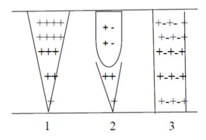
In the above diagram figure 1 indicate formation positive space charge tending towards cathode. Figure indicates how field of positive space charge ionizes the gas. Figure indicates formation of avalanche between plates.
