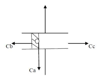
This type of discharge mainly occurs due to presence of internal voice or cavities. If solid insulation consist of voids which may be considered as gas pockets, when the high voltage is applied to such a insulation ionization process occurs in the gas pockets which may leads to internal discharge. This internal discharge may be treated as partial discharge. If the structure of solid insulation consists of multiple voids then possible multiple partial discharge may occur.
